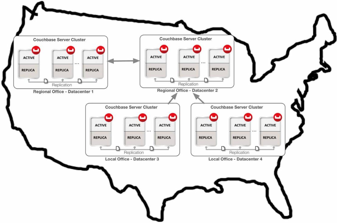
Figure 7: Using bidirectional and unidirectional replication to selectively replicate data between datacenters
